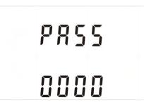
Setting up is password-protected so you must enter the correct password (default '1000') before processing.
