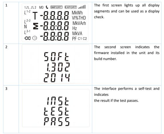
\*After a short delay, the screen will display active energy measurements.
