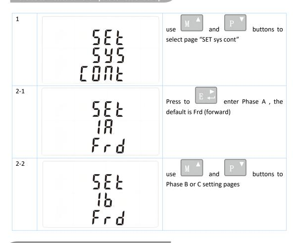
How to operate if phase A is reversely connected
