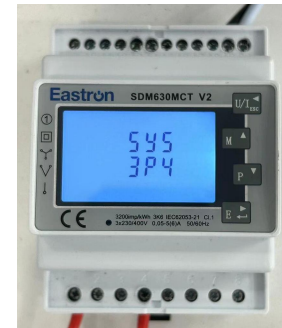
5. Press P button to select SYS, and press E button for 3s to enter SYS setting interface
