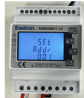
4. Press E button for 3s to enter the setting interface
