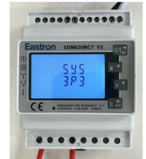
6. Press P button to select 3P3, then press E button for 3s to exit SYS setting, then press U/I button for 3s to exit the initial interface.
