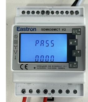
2. Press E button for 3s to enter the password input interface
