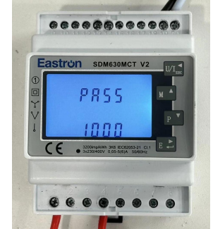
3. Press M button to enter the password (default 1000)
