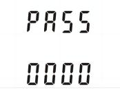
Setting up is password-protected so you must enter the correct password (default '1000') before processing. If an incorrect password is entered, the display will show: PASS Err
